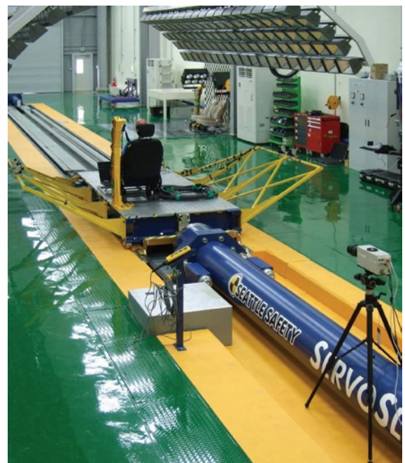
Easily conduct whiplash testing on ServoSled.
